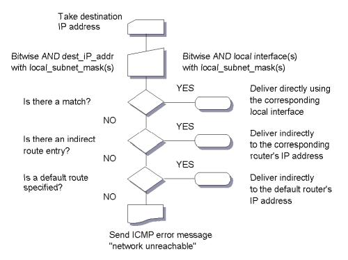
Figure 25. IP Routing Algorithm (with Subnets)
