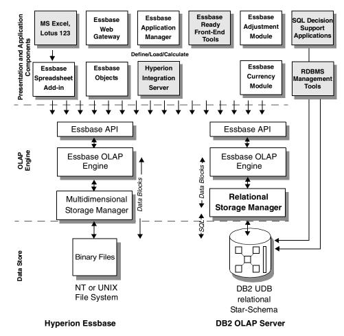
Figure 13. Hyperion Essbase and DB2 OLAP Server Architectures
