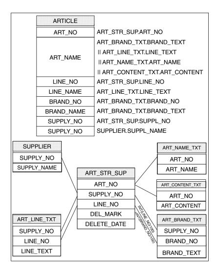
Figure 36. Dimension Table PRODUCT from Join of Intermediate Sources
