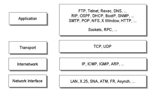
Figure 17. TCP/IP Architecture Model: Layers and Protocols
